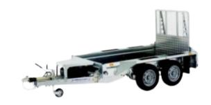
We run various sizes of plant trailers with gross weights of 2700kg - 3500kg, they all have fold-down ramps.
